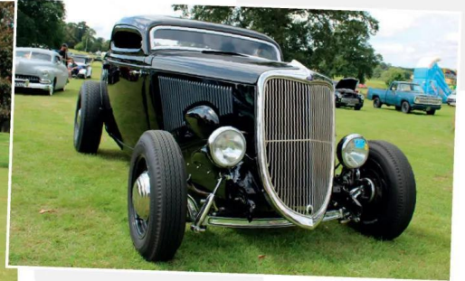
Steve Young's Hemi-powered '33 Ford received a hefty roof chop at Buckland Automotive earlier this year, with louvred bonnet sides and a rear pan being added at the same time. The coupe was selected as both Traders' and Lucky's Hot Rods / Mad Fabricators' Picks
